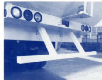
Under-ride protection meets FMVSS requirements.
