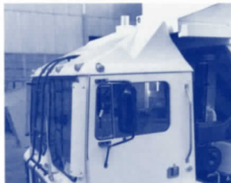
Optional lightweight cab protector has built-in light package.
