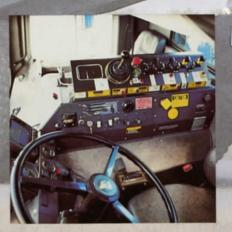
CAB MOUNTED CONSOLE features airactuated hydraulic controls. Many select options such as Auto-pack and a variety of vision systems are also available.
