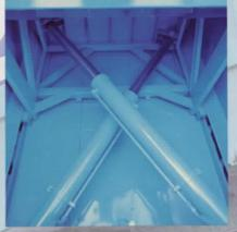
PURE PACKING POWER from crossed, single stage/double-acting cylinders. Simple, low-maintenance and long lasting.
