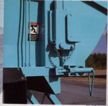
HYDRAULIC TAILGATE LOCK/UNLOCK assures positive locking and sealing.
