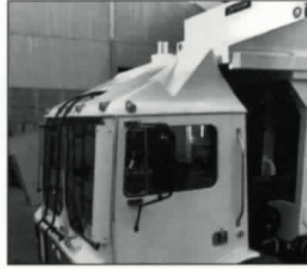
Optional lightweight cab protector has built-in light package.
