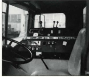
Cab-mounted console features "featherable" air controls.
