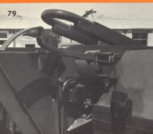
Retaining springs prevent container from slipping under icy, slick conditions.
