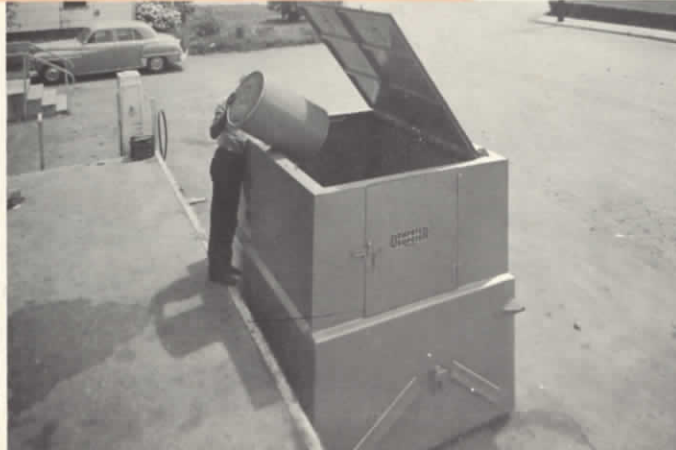
Photo 18. Ten cu. yd. Universal Container being loaded from dock.
