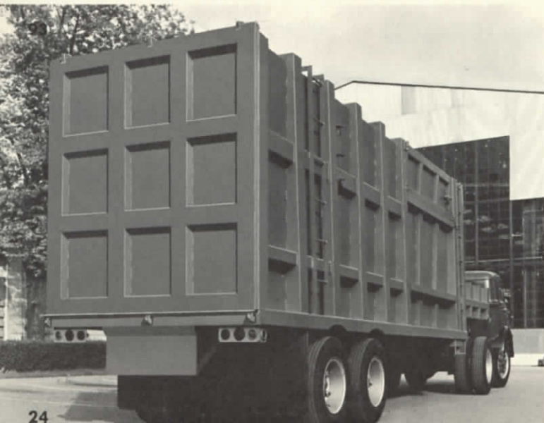
Shown below is the Model DB-53, which is 12 ft. 6 in. high and has a storage area of 53 cu. yds. of compacted material.
