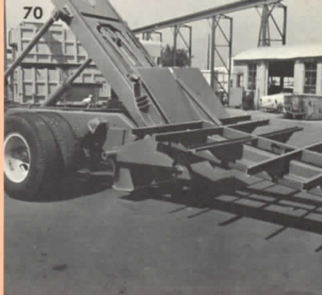
Bail engages first hook station and container base is pulled up on tipping frame.
