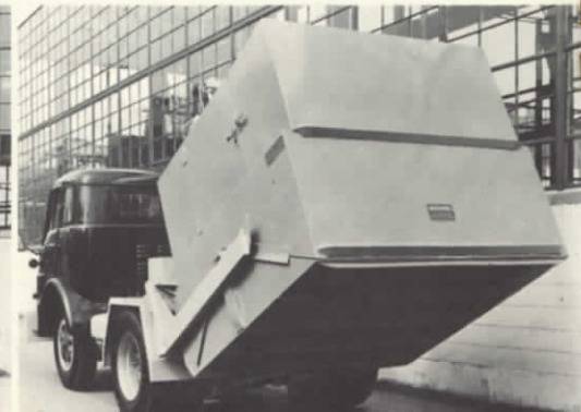
Photo 44. With container in carrying position, GRD moves toward trailer or disposal area.
