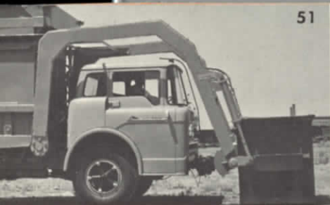
Truck approaches Dumpmaster container and forks engage lifting channels on the side.
