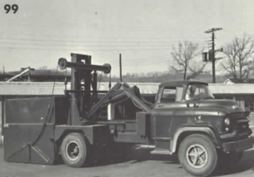
In photo below, DTLF is backed up to container and lifting links are attached.
