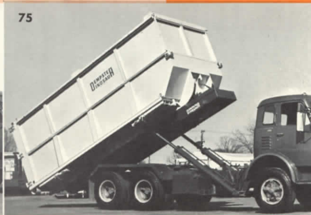
Bail cylinder pulls base up on tipping frame which is then lowered.
