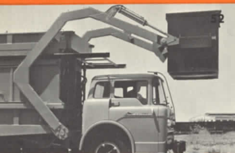
Container is raised off ground as lifting arms rotate backward.
