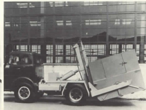
Photo 43. Container is lifted up the skid frame.
