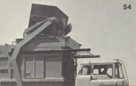
Container inside hopper opening. Top lids swing open and refuse is emptied into compaction body.
