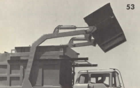
Container begins to tilt backward as it approaches the hopper opening.
