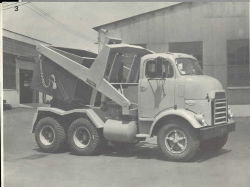
Shown above is the DEMPSTER-DUMPSTER LFW 503-C , mounted on a tandem chassis. This model has a capacity of 15,000 lbs. and is used for handling dense, heavy materials.
