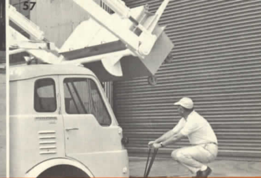
Outside controls are provided for use when driver must dismount to go inside or to inaccessible spots to move container to lifting forks.
