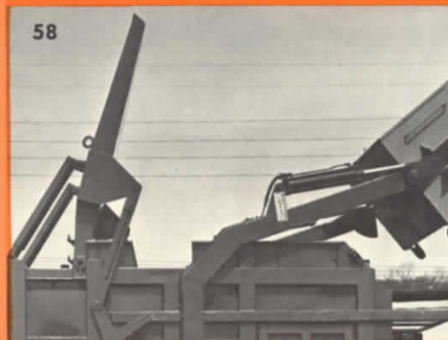
An optional automatic hopper cover increases body capacity by permitting use of the hopper area.
