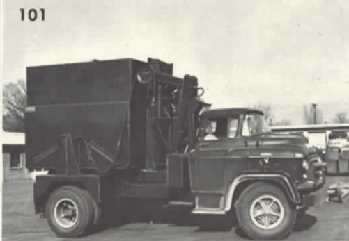
Scissor-hinged cylinder retracts, pulling container into carrying position.
