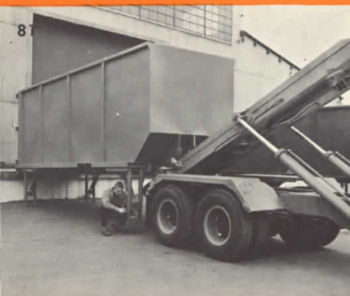
To leave containers at dock height adjustable-height legs are used.
