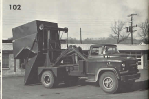
Container has been moved to the rear and is shown in dumping position.
