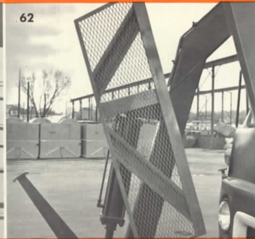
Movable hopper extensions are for use in windy areas. They are secured to clearance arms, as shown above.
