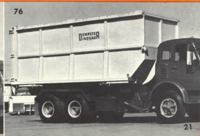
Bail cylinder pulls base up on tipping frame which is then lowered.
