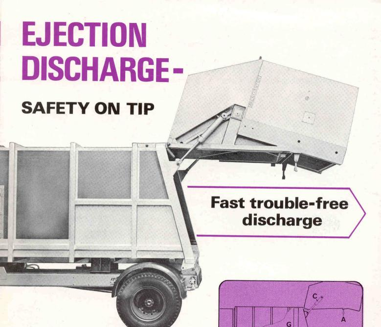
The ejector discharge gives rapid clean emptying of the body whilst the large capacity hopper and the power of the packer plate gives an unequalled loading rate - 1.4 m . in 12 seconds, compressed with a force of 45 tons.
