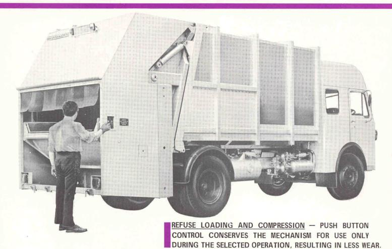
BULKMASTER is a two stage automatic hydraulic compression loader with dual crushing action, which not only handles bulky refuse at speed, but gives uniform density of load throughout the body.
