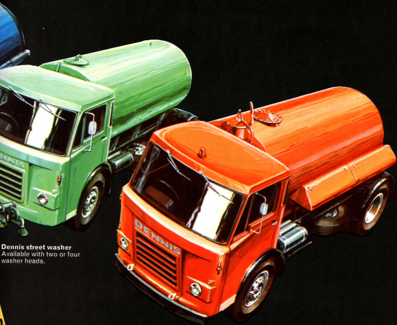
Dennis cesspool emptier Available in 800 (3636-77 litre) 1000 (4545-96 litre) or 1500-gallon (6818-94- litre) capacity.
