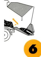
The swivel compression plate also then retracts and another cycle is started as in diagram 1.
