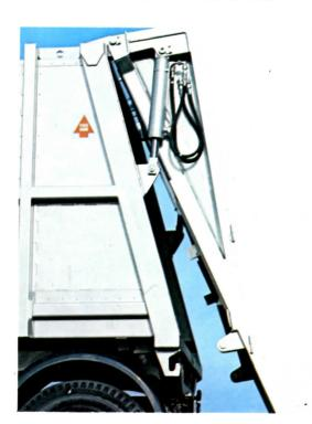
The Loading Hopper Unit is of typically meticulous Dennis design. It is a jig built all-welded framework of steel section, corrosion protected as is customary with Dennis vehicles.
