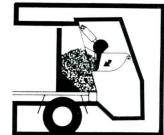
With vehicle in position at disposal site, hopper locks are automatically released.
