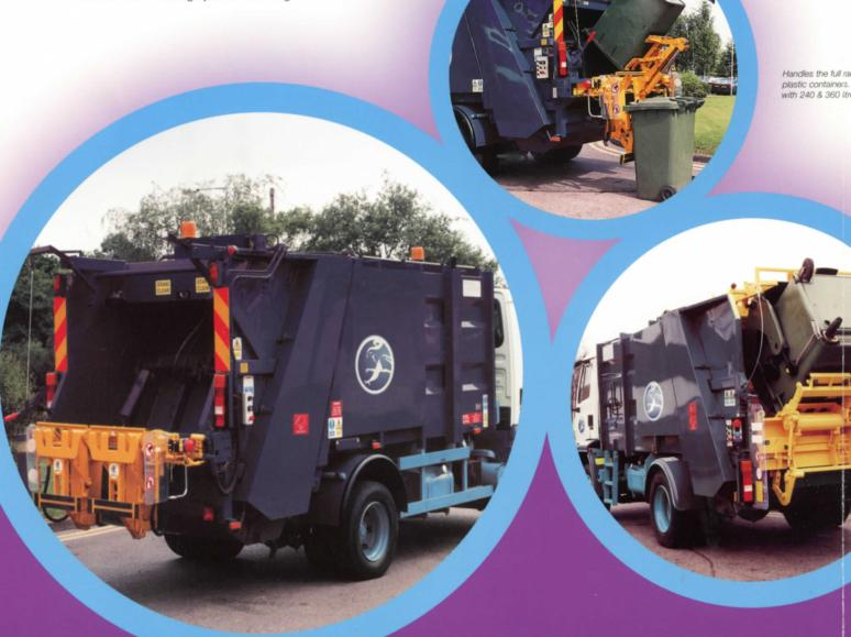
Slide cylinders mounted externally avoids damage and enables easy maintenance.
