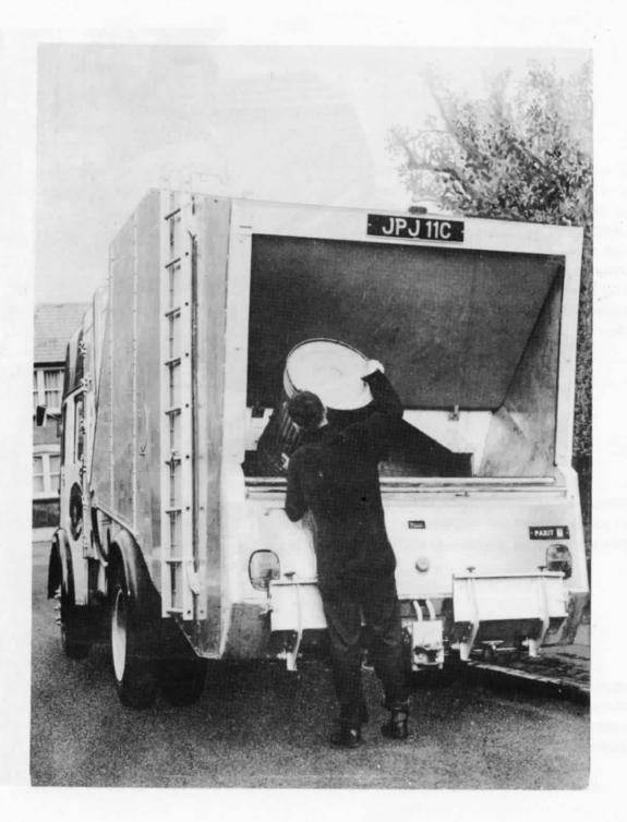
Attention is drawn to the low loading height, generous ground clearance, inset stop and tail lights, folding loaders' steps and the hand rail. The hinged fibre-glass flap can be used as a cover for the loading aperture or as a dust screen which is moved by the action of emptying a bin. Access to the large salvage well is by the folding ladder on the nearside.
