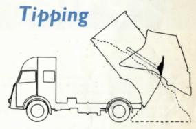
Twin hydraulic rams with an automatic overload device operate the tipping of the body. The hopper is anchored by a restraining chain which passes over the roof of the body and is attached to the chassis aft of the driver's cabin.
