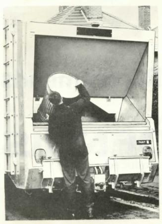
The Dennis 25/40 cubic yard Paxit IIIA or 35/50 cubic yard Paxit Major IIIA with continuous loading two stage compression mechanism can deal quickly and efficiently with bins for normal manual collection. The design enables the vehicles at a later date to be modified as necessary to stage 2 or 3, allowing the gradual introduction of dustless loading to take place within the authority.
