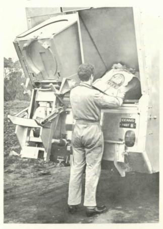
The Dennis Paxit fitted with one dustless shutter for use with hinged lid bins, leaving space at one side for manual loading, normally used where a pilot scheme is operating in an area which is not completely dustless.
