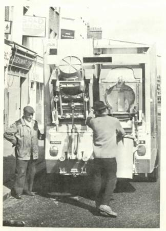
The Dennis Paxit equipped with two dustless shutters for use in a completely dustless area. using the lightweight Dennis plastic bins, a high rate of loading can be achieved without fatigue to the loaders, litter in the wake of the vehicle or damage to the bins.
