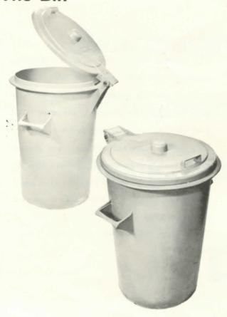
The Dennis hinged lid bin is made from Polypropylene. It is injection moulded giving thickness and strength where needed. The handles are an integral part of the bin and the lid cannot be removed or"lost", ensuring that the refuse is kept dry.
