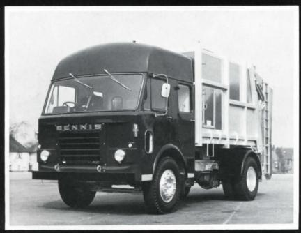
"Automatic loading compression type refuse-collector" (With ejection discharge)
