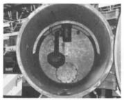
SYPHON DEVICE A floating syphon pipe is fitted in the sludge compartment for drawing off excess water to leave a dry load of sludge.
