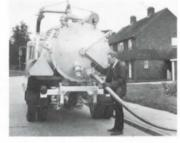
CESSPOOL EMPTYING EQUIPMENT Cesspool Equipment 3" (76·2mm) inlet and outlet valves and one hose
