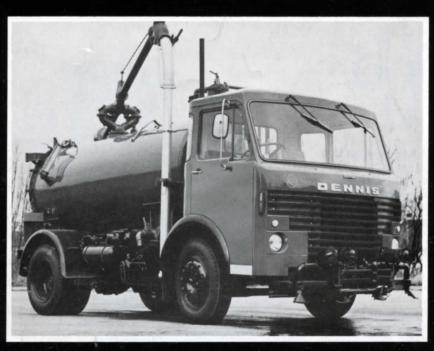
Vacuum principle gully emptiers for efficiency & versatility
