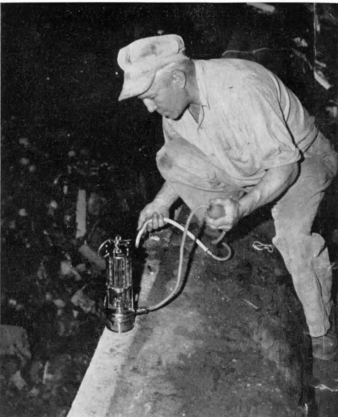
Testing air in an incinerator pit to assure safety of men working in it. Oxygen deficiency will cause lamp to go out. If explosive gases are present, flame will change color and burn brighter.
