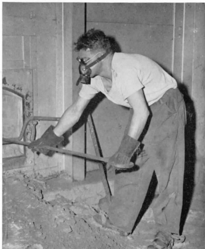
Incinerator laborer cleaning soot chamber protected against dust by goggles and respirator. He wears wooden sandals to prevent feet being burned by hot soot.
