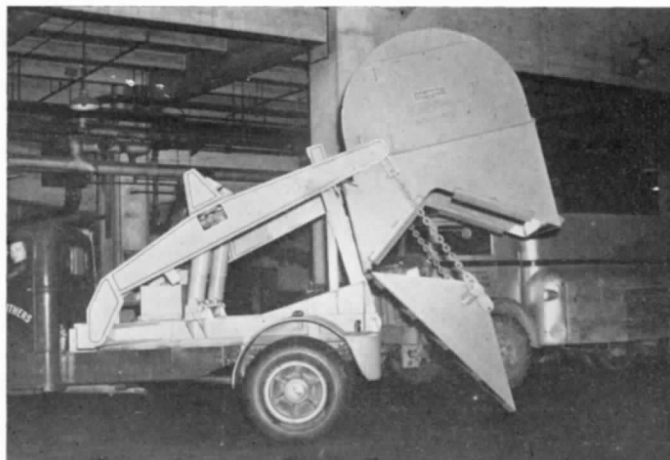
Detachable container unit to be employed in markets, hospitals, school areas, etc. Containers hold 10 and 12 cu. yds. of refuse. Cost: Chassis, $4,500; hoist, $3,100; container, $800.
