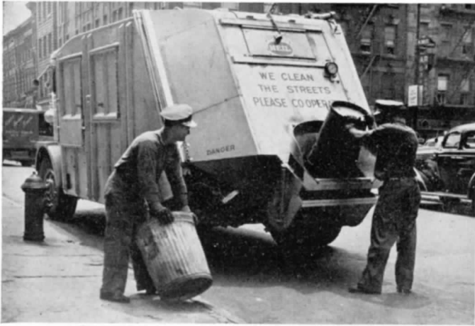
A demonstration unit of the Baldt-type loader, designed by a member of the Department's motor maintenance bureau. Simplicity of design and ability to handle non-compactables such as ashes may make this compactor a valuable addition to the Department's fleet of trucks.
