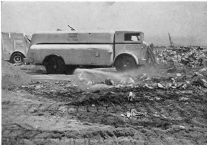
Flusher truck sprays refuse with disinfectant.
