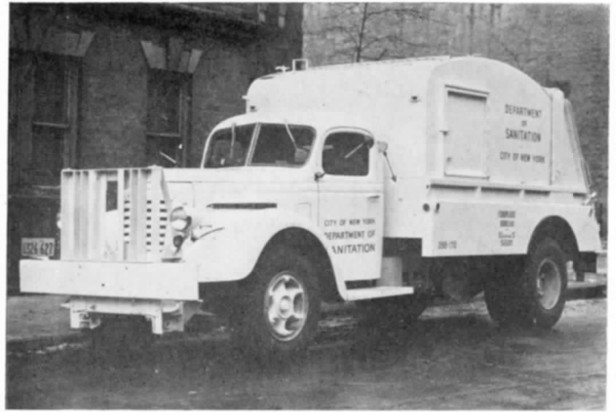
New 15 cu. yd. compactor collection truck which compresses about twice the capacity of mixed refuse as conveyor and hand-loaded vehicles. Cost: $7,860.
