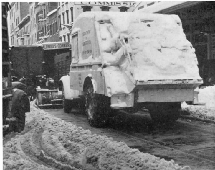
Plow-equipped refuse collection trucks serve a double purpose during the snow season.
