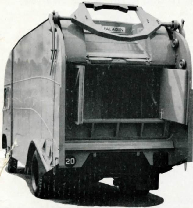
This rear view of a Compressmore fitted with the "Paladin" bin-lifting mechanism shows the rear doors of the body open and the bin lifter itself raised clear.
