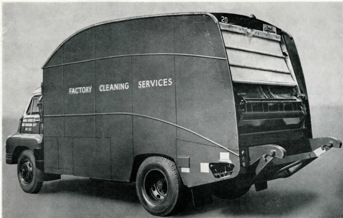
This rear view of a Compressmore with industrial bin-lifting attachment shows a body exterior panelled in aluminium and painted. This particular vehicle is one of a fleet of Compressmores in regular use at the Vauxhall Motors and Bedford Truck factories at Luton and Dunstable. Large capacity wheeled bins are used as refuse receptacles, and these containers are emptied into the vehicle at numerous refuse collection stations throughout the factory areas. All operations can be controlled and handled by the driver alone. See details of bin-lifter on page 4 of this folder.
