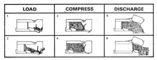
from two hydraulic rams situated on the roof top. The lower barrier is fitted with twelve teeth which grip and shred the refuse as it is transferred to the main body. This action breaks down cardboard and wooden boxes and effectively shreds sacks. Due to the design of the hopper and compressing barriers, there is no necessity for seals as the action is self clearing.
