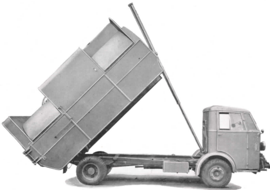
Shows the body tipped, giving a large angle for discharge.
