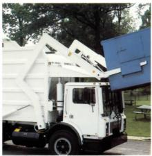
Hercules' Lift Arms are engineered for extremely level container handling made easy and fast—cycle time is a quick 20 seconds.
