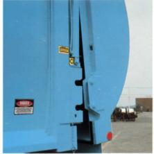
Automatic lock/unlock rear door is an exclusive E-Z Pack ease of operation and safety feature. Assures positive locking and sealing; eliminates manual turnbuckles.
