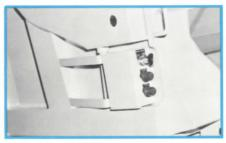
Push Button Control System — electrically actuated for either automatic cycling or manual operation. Packer plate can be stopped or reversed at any point in cycle.
