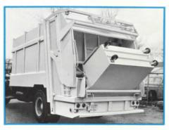
Conventional 1 yard and dock type 2 yard container systems are available with E-Z Pack RL. Just hook chains to packer plate cylinder base and activate packer for fast, easy, no spill dumping. Simple but sanitary collection.
