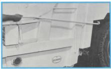
Manual Back-up Control System — provides packer plate manual operation by hydraulic power. Hooks up quickly and easily and is operated from curb side of Hopper.
