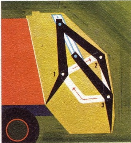
Fully-Automatic Packer Blade Cycle —(1) Packer blade is at full-forward position. (2) When actuated, it rides track over hopper, (3) passes hopper lip and sweeps refuse into body. Packer blade stops at full-forward, forcing load against ejector blade. Blade can be completely reversed at any point during packing cycle.
