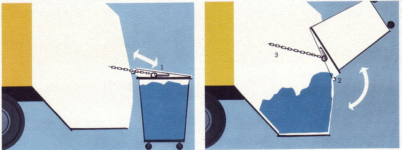
Easy Containerization —1 and 2 cu. yd. containers can be quickly and easily dumped. All you do is—(1) attach chains. (2) Body-stops catch container trunnions. (3) Packer blade moves to full-in position and dumps container. Back down is just as easy.
