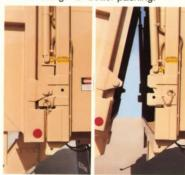
With the cylinder in retracted position, the tailgate is locked. Lifting, extension lowers locking mechanism to unlock.
