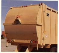
Three basic body sizes - 26, 31, and 36 yards - are available. By adding the one or three cubic yard bubble tailgate, you may have a 27, 29, 32, 34, 37 or 39 yard side loader. A 29 yard is illustrated, a 26 yard body with a 3 yard tailgate.
