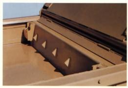
One-piece ram with in-line cylinders push into body, reduces hopper wear and maintenance. Load retention ledge reduces spring back of trash. No ram hinge or tracks to bind ram. Metal hinged scraper bar.
