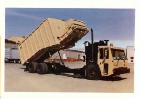
The E-Z Pack® unitized design eliminates the leakage, spillage and potential seal wear found in two-piece body designs. It dumps quickly, cleanly and safely. Compactor can be cycled while unloading to clean out hopper and body.
