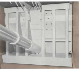
E-Z TO PACK: Heavy duty packer plate compresses each load . . . tightly . . . with a simple outside control. There's no lost space either. The scientifically designed plate packs the body full: top, corners, sides, and bottom.
