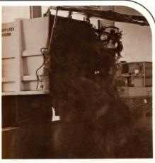
E-Z TO EJECT: One lever releases all six tailgate latches, another hydraulically raises the tailgate up out of the way. Then that packer plate pushes everything out. Everything! And you're always on a solid foundation . . . There's no raising the body to dump.
