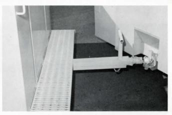
**HEAVY DUTY TRAILER HITCH.** Side opening type, with rear ball hitch recessed—"T" lift bar insures easier handling and is standard equipment.
