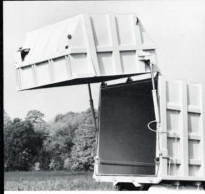
Bubble Tailgate lifts up and clear for Quick Discharge of load.
