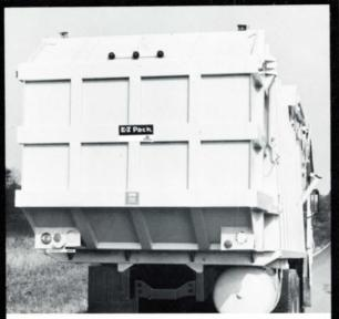
All tailgate mounted lights raise clear when unloading. All wiring is fire resistant.
