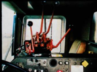
Smooth cable control makes lift operations simple. For convenient driver access, all tailgate and ejection controls are located in the cab.
