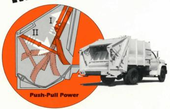
Peabody's combination push-pull leverage. Smooth and powerful! A dual cylinder system delivers direct packing thrust into the compaction cycle. This patented engineering design works at peak efficiency through years of heavy use.
