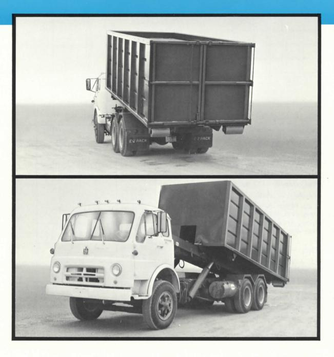
E-Z PACK OPEN TOP ROLL-OFF CONTAINERS are ideal for demolition jobs — just spot a convenient container close to clean up areas. Eliminates tying up several expensive Dump Trucks, by allowing one Tilt Frame Truck to handle a number of containers. Good for incinerator ash removal, collection of noncompactible refuse, wood, stone, etc. Containers can be loaded by hand, hopper chute or front end loaders. Can also be used to accumulate scrap metal for salvage.
