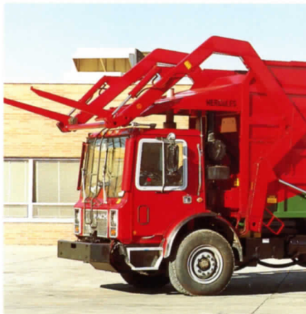
Hercules' Lift Arms are engineered for extremely level container handling made easy and fast—cycle time is a quick 20 seconds. Available with 6K, 8K or 10K arms.
