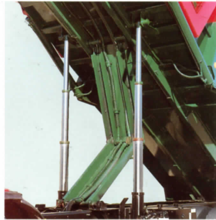
Exclusive E-Z Pack under-body stabilizer helps keep the unit from swaying during off-loading. The stabilizer also provides a shortcut for the body hydraulics, eliminating the need for hoses and fittings the full length of the chassis and back up the body.
