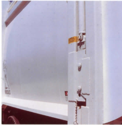
Curved body design of abrasion resistant steel has a higher strength-to-weight ratio than flat, braced walls. The outside surface sheds the elements while the inside surface eases off-loading.
