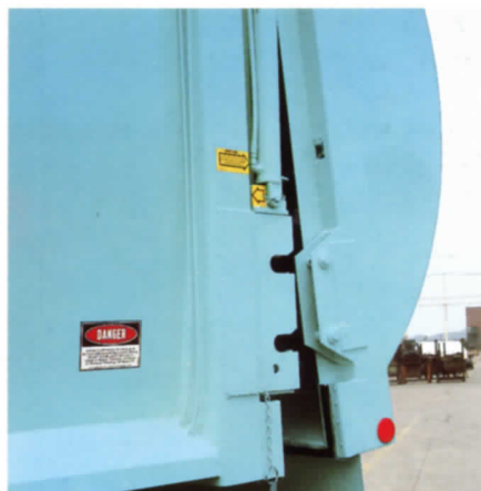
Automatic lock/unlock rear door is an E-Z Pack productivity and safety feature. Assures positive locking and sealing; eliminates manual turnbuckles.
