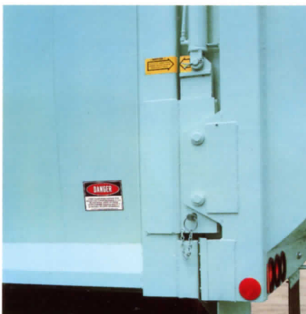
Automatic lock/unlock rear door is an E-Z Pack productivity and safety feature. Assures positive locking and sealing; eliminates manual turnbuckles.
