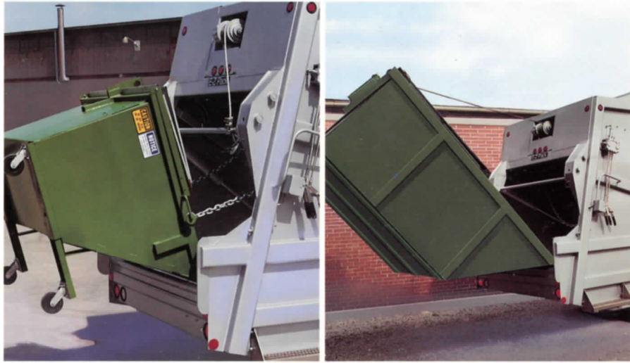
Can dump 1-3 yard containers in one cycle, saving time. Empties large containers fast due to high container dump angle. Container lid swings free and out of the way—doesn't catch refuse, dumps cleanly.
