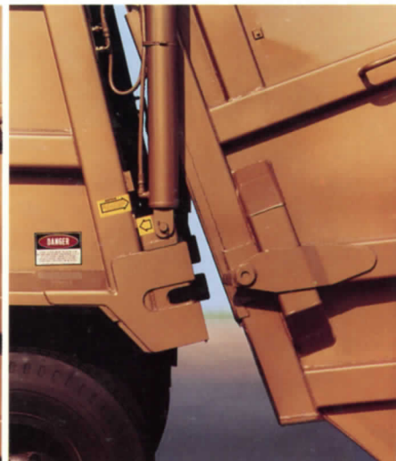
Automatic lock/unlock tailgate is an exclusive E-Z Pack ease of operation and safety feature. Assures positive locking and sealing; eliminates manual turnbuckles.
