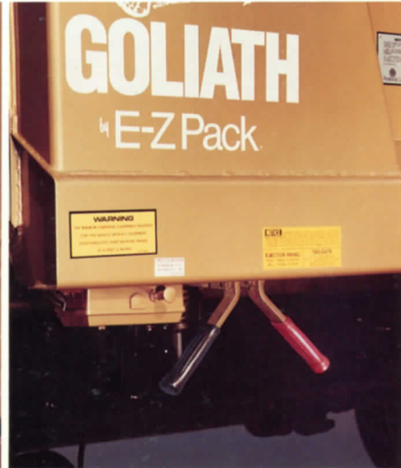
Single control lever for the automatic lock/unlock tailgate allows the operator to maintain a safe distance at all times during the off-loading procedure.
