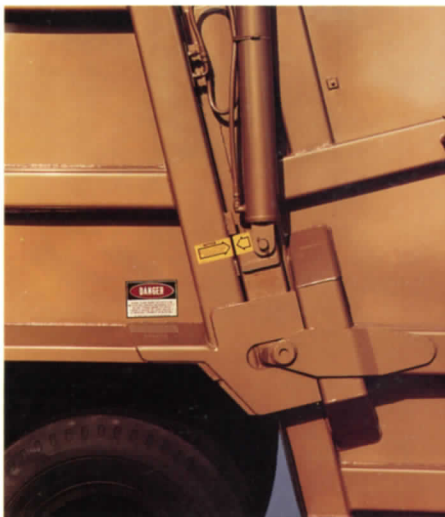
Automatic lock/unlock tailgate is an exclusive E-Z Pack ease of operation and safety feature. Assures positive locking and sealing; eliminates manual turnbuckles.
