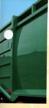
Curved sidewalls — high strength-to-weight ratio; no heavy cross members; sheds elements — extending service life; eases off-loading.
