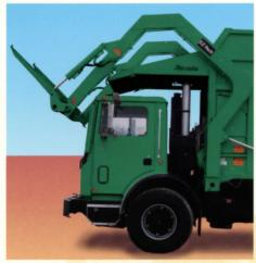
Lift Arms — are engineered for extremely level container handling made easy and fast—cycle time is a quick 20 seconds. Available with 6K, 8K or 10K arms
