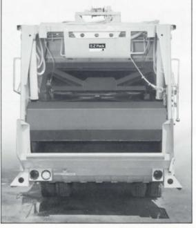
The C-250 manually operated Rear Loader gives you the capability to handle large volume containers—up to 10 cu. yds., big commercial and industrial stops as well as longer residential routes where volume and dense compaction pay off in profitability.
