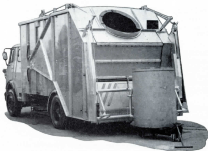
50 cub. yard BINLIFT Model WITH 1\frac{1}{4} cub. yard CONTAINER IN POSITION READY FOR LIFTING
