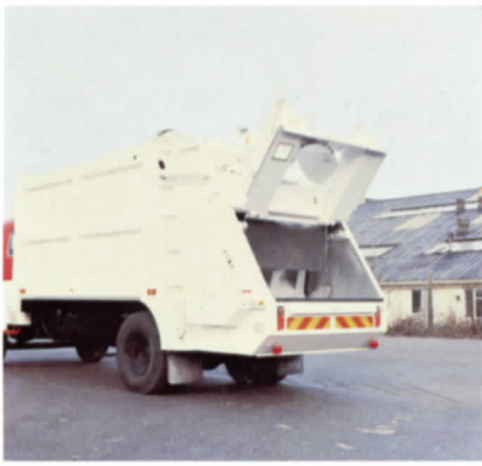
Bin lift equipment stowed
