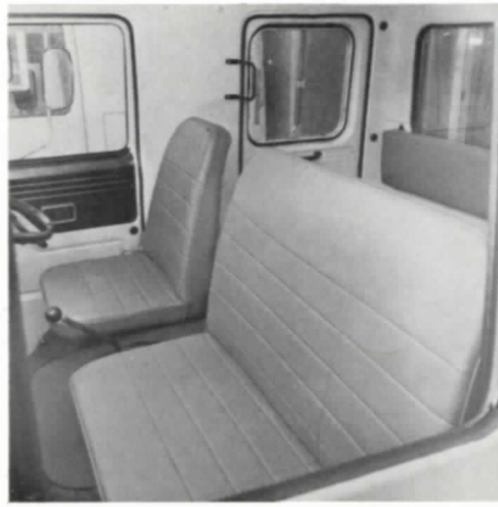
Interior of a crew cab which can accommodate up to seven men (including the driver) and any necessary equipment without impeding the driver in any way.
