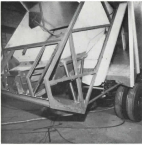
This uncompleted canopy shows the position of the canopy safety prop in use (common to both models) and the accessibility of the 'Musketeer's' impeller screw gearbox.
