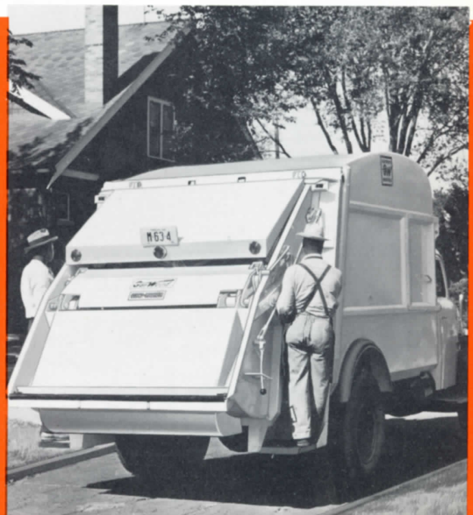
Large safety riding steps mean less walking between pick-ups. Reduces crew fatigue.
