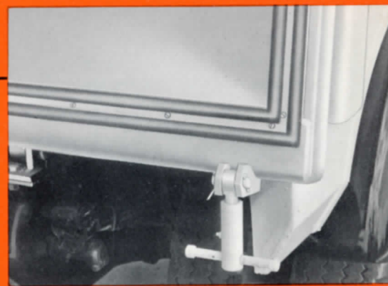
Double tubular tailgate seal prevents odorous fluids from dripping onto street.
