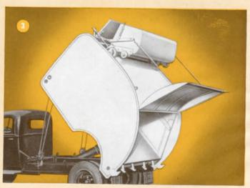
the hatch, the cover of which automatically opens and closes.
