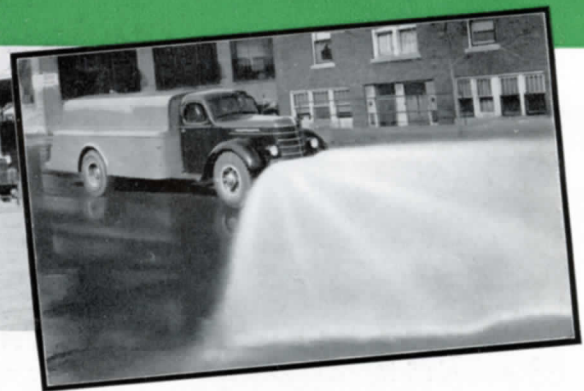
Fig. 14 (above, right)—Sprinkling attachment. Adjustable brass horizontal sprinkling heads or nozzles installed at front (or rear, optional). Cab control.
