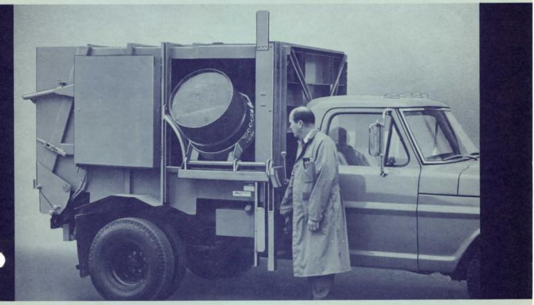
Here's a fast, positive method to dump heavy refuse trash barrels into a Gar Wood Load-Runner, a trash body, or other applications.
