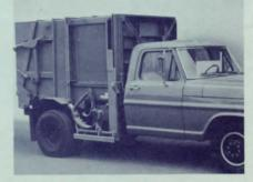
When on the road the lift attachment tucks up and out of the way. Hydraulic cylinder is enclosed for protection.
