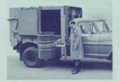
Operator activates hydraulic valve to raise barrel. The valve permits starting or stopping the barrel in any position.
