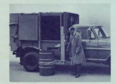
Barrel is securely held by spring loaded chain lock. Belting protects the finish of the container.
