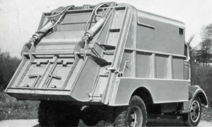
3 Doors are closed when the loading trough is full. Notice how the trough slopes out, in the best position for loading.
