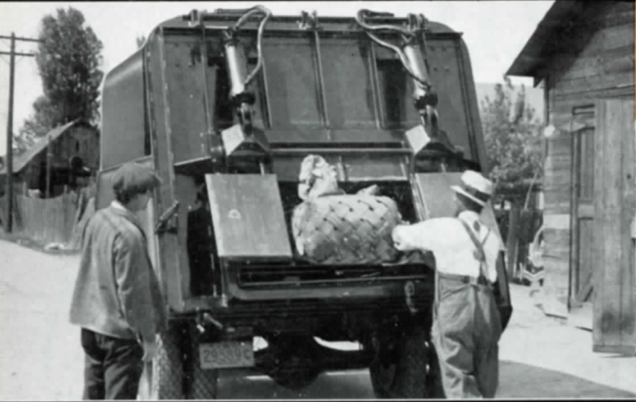
1 Doors are swung back for loading. There is room for cartons, boxes and bulky trash in the loading trough, which is almost as wide as the body.
