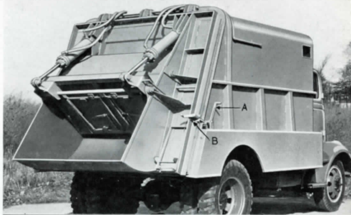
4 Compressing load by means of two hydraulic cylinders which operate the "ram". This action also cleans out the trough in readiness for another filling. (A) Lever to operate ram. (B) Tailgate locking device.
