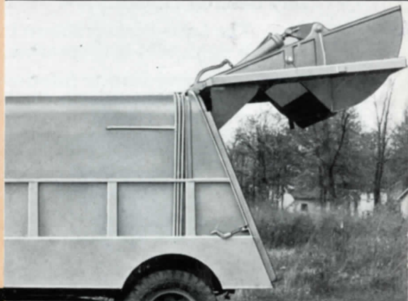
6 Rear end gate can be raised at any time, by means of the two cylinders located inside the body so that cartons, crates and other bulky objects can also be loaded.
