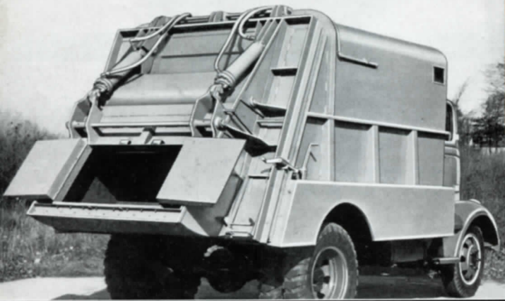
2 Notice the low height (30" to 40") of the loading edge from the ground. This accessibility means faster, easier loading and eliminates risk of injuries.
