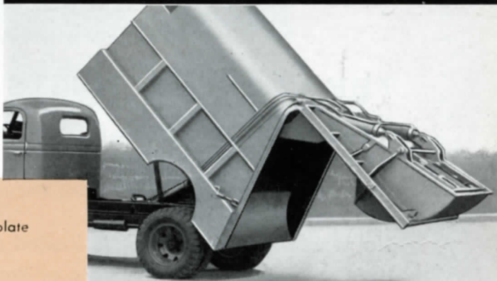
4 Compressing load by means of two hydraulic cylinders which operate the "ram". This action also cleans out the trough in readiness for another filling. (A) Lever to operate ram. (B) Tailgate locking device.
