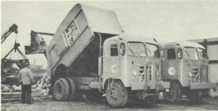
Chicago's Bureau of Sanitation has added 50 of these combination International R-212 trucks and Gar Wood Load-Packer bodies to its refuse collection fleet.
