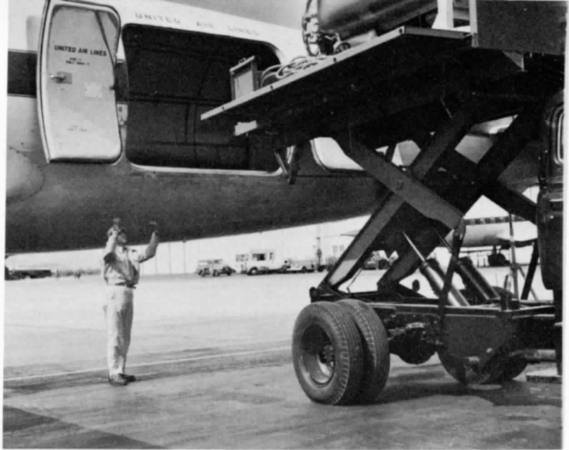
A Gar Wood-St. Paul Hi-Lift hoists freight aboard a United Airlines plane in San Diego, California. United also uses Hi-Lifts for handling passenger food trays.
