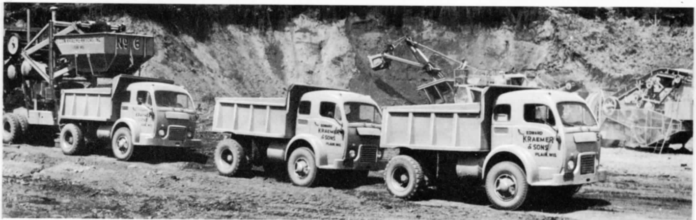
Part of a fleet of 55 Gar Wood-St. Paul hoists and bodies, owned by Ed Kraemer & Sons, Plain, Wisconsin.
