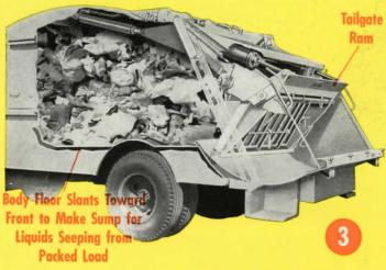
3. The tailgate ram is actuated by two heavy-duty hydraulic cylinders that provide a total force of from 50,000 to 70,000 pounds (depending upon Load-Packer size) . . . more than ample to compress the contents of the hopper into the body. At end of ram stroke, the retaining plate automatically latches into its original position to hold the compressed body load. The tailgate ram then automatically returns to loading position (see page 3).
