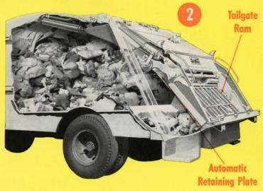
2. When hopper has been filled and loading door closed, the tailgate ram begins its movement (see also page 3). At that instant, the retaining plate is automatically released and snaps back against the tailgate.
