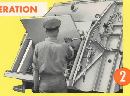
To empty the closed hopper into the body of the Load-Packer, the crew member just presses a button (as illustrated at right). The hydraulically operated ram then forces the refuse into the body where it is held in place by an automatic retaining plate (see page 5). If the body is full, the ram stops automatically and prevents damage from overloading.
