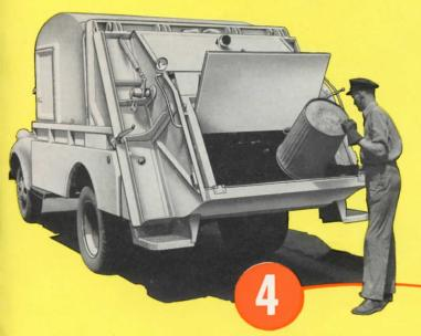
When the hopper has been emptied, the ram automatically returns to its original position and the loading door opens automatically. Without any action by the crew, the hopper is now ready to be filled again. Only 15 seconds elapse from time the full hopper is closed for emptying until it is open again for the next load.
