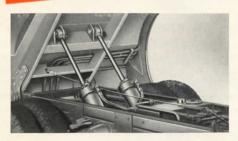
Shown here are the two hydraulic hoists under the body of the Load-Packer that are used only for dumping the load...they have complete control of the body throughout entire lifting, holding and lowering cycle. These twin hoists assure better distribution of the load when dumping and minimum stress concentration in both the body and the chassis.
