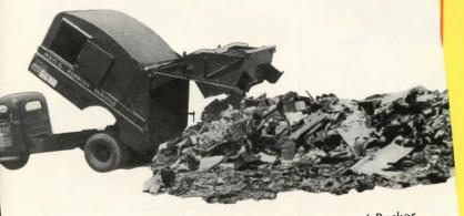
There are no obstructions on the inside of the Load-Packer to interfere with clean and complete dumping. Twin underbody hoists (used only for dumping) powered by a large body hoists (used only for dumping) powered by a large capacity Gar Wood pump assure fast dumping of the load.
