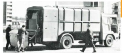
HALLER COMPACTING COLLECTOR emptying 1.1 m 3 refuse containers.
