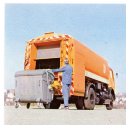
Lifting mechanism for refuse containers of 1.1 m 3 content.
