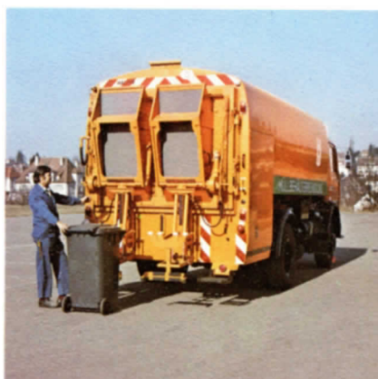
Double lifting mechanism for refuse containers of 220 litres content.
