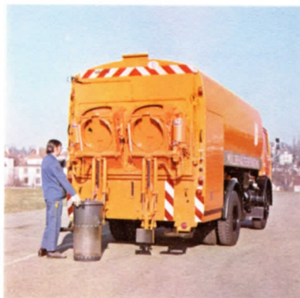
Double lifting mechanism for refuse bins of 110 litres content.
