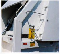
The FORMULA 5000 rear loader combines solid quality, full seamless welded high tensile steel construction, with advanced design high pressure cylinders. The reduced body weight lets you pack a greater legal payload into the industry's most desirable rear loader.
