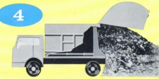
At disposal point, operator simply raises tailgate, flips ejection control—and ejection plate pushes tightly compacted load out of body.
