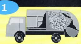
At start of collection route, ejection plate can be positioned at rear of body. Packer plate then forces first loads against ejection plate.
