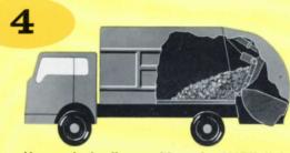
Hopper in loading position, the MARK II is ready for another load. Packer plate remains in forward position, holding refuse securely in body. Entire cycle is complete in 12 seconds!
