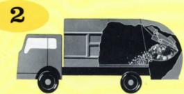
Packer plate meets hopper at top position, starts to bulldoze refuse forward into body with rolling action that wipes hopper clean.
