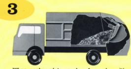
When packer plate reaches forward position in packing cycle, hopper returns to loading position. Safety door automatically moves up.
