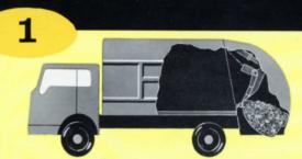
When hopper is full, operator pushes button to start loading cycle. Packer plate automatically moves back and upward as hopper rises. Safety door (optional) covers load opening.
