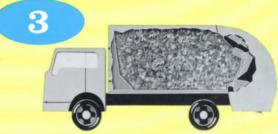
With body completely full, entire load is uniformly compacted between packer and ejection plates. "Duo-Press" compaction from first to final loads assures full capacity each trip.
