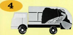
Hopper in loading position, the MARK III is ready for another load. Packer plate remains in forward position, holding refuse securely in body. Entire cycle is complete in 12 seconds! REVOLUTIONARY
