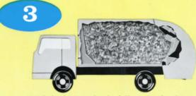
With body completely full, entire load is uniformly compacted between packer and ejection plates. "Duo-Press" compaction from first to final loads assures full capacity each trip.
