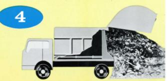
At disposal point, operator simply raises tailgate, flips ejection control—and ejection plate pushes tightly compacted load out of body, in one powerful, smooth stroke.
