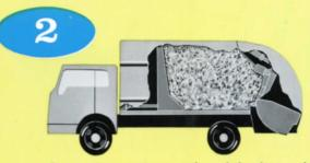
Compaction continues with each loading cycle, squeezing material between packer plate and ejection plate, until hydraulic relief valve allows ejection plate to move forward in body. No operator attention required.
