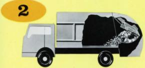
Packer plate meets hopper at top position, starts to bulldoze refuse forward into body with rolling action that wipes hopper clean.
