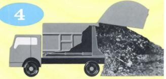
At disposal point, operator simply raises tailgate, flips ejection control—and ejection plate pushes tightly compacted load out of body.
