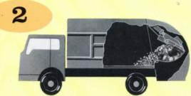
Packer plate meets hopper at top position, starts to bulldoze refuse forward into body with rolling action that wipes hopper clean.
