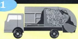
At start of collection route, ejection plate can be positioned at rear of body. Packer plate then forces first loads against ejection plate.
