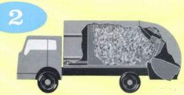
Compaction continues with each loading cycle, squeezing material between packer plate and ejection plate, until hydraulic relief valve allows ejection plate to move forward in body.
