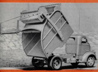
**EASY TO DUMP LOAD** — Body raised to 45° angle in twelve seconds. Tapered construction of body assures quick, clean disposal.
