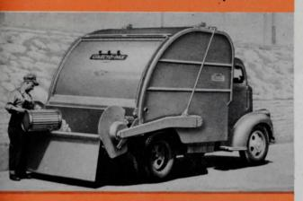
**EASY TO LOAD** — 35" loading height makes the work easy for your crews. Hinged lid covers loading bucket.
